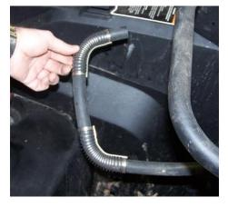
12) Attach heater hoses to heater core as shown below.
