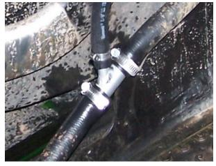
9) Repeat step 8 on radiator hose located above driver's side front wheel. Note Y-Adapter orientation. Attach and route longer heater hose through center of vehicle and out through passenger side "foot well" area. Elevate hose and keep together with previously installed heater hose. Using 2 or 3 zip ties, secure hoses to vehicle to prevent chafing.
